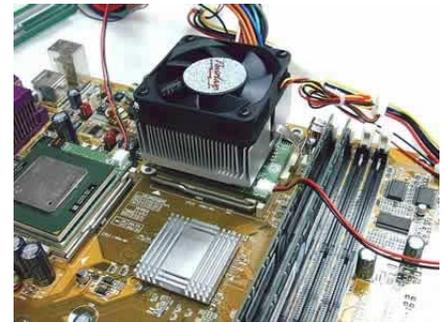
The PowerLeap heatsink and fan installed on the PL-370/SMP.
