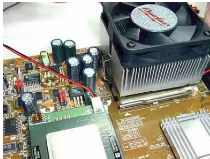
The PowerLeap heatsink and fan installed on the PL-370/SMP.
