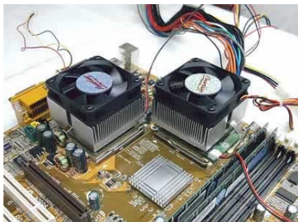
A PowerLeap heatsink and fan installed on each PL-370/SMP.
