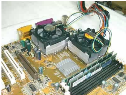
The original processors (with installed heatsinks and fans).
