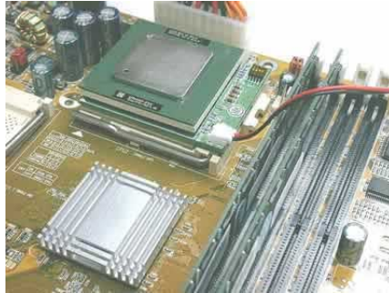
The PL-370/SMP installed in a processor socket.
