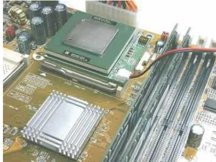
The PL-370/SMP installed in a processor socket.
