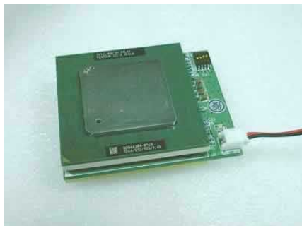
The PL-370/SMP with connected power cable.
