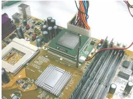
Inserting the PL-370/SMP in a processor socket.
