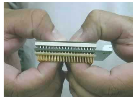
Making certain the processor is firmly inserted into the PL-370/SMP.
