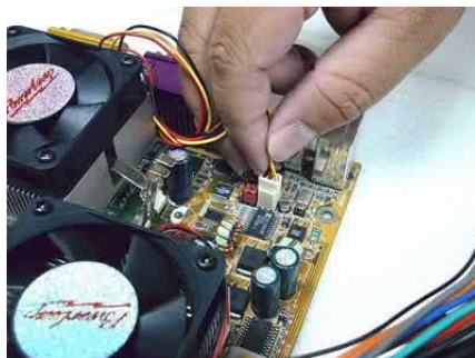
Connecting the power cable for the PL-370/SMP's fan to the motherboard.
