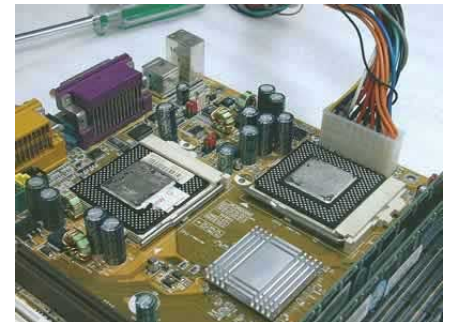
The original processors after removing the heatsinks and fans.
