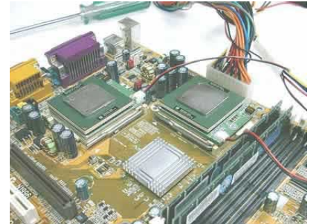
A PL-370/SMP installed in each processor socket.
