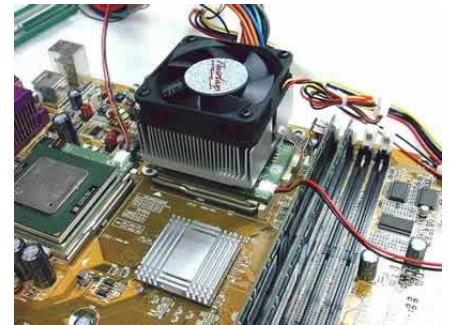
The PowerLeap heatsink and fan installed on the PL-370/SMP.
