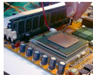
Install the PL-370/T™ into the ZIF Socket
