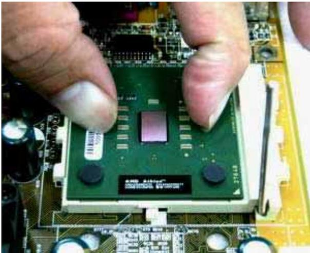
**Important:** Make sure that there is no "space" left between the AMD CPU and the PL-AXP adapter. A poor "connection" may prevent the PL-AXP from working correctly.
