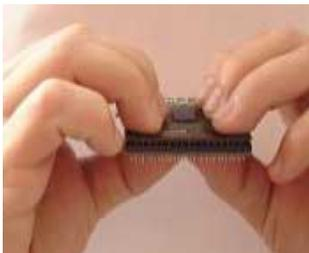
Insert a New CPU into the PL-Neo/T™
