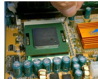
Insert the PL-Neo/T™ into the ZIF Socket
