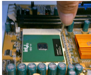
Lift the arm of the Socket to remove the old CPU
