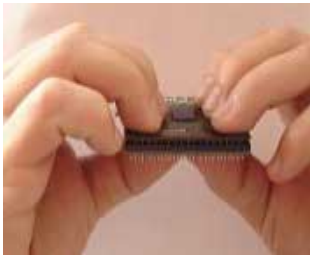
Insert a New CPU into the PL-Neo/T™
