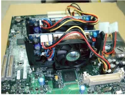
Inserting the second PL-P3/SMP into the processor slot.
