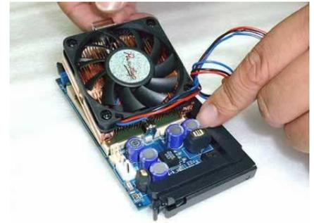
Installing the heatsink/fan onto the processor.
