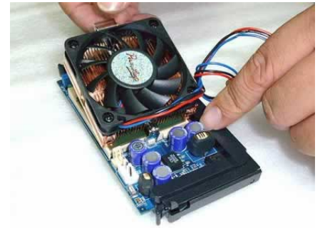
Installing the heatsink/fan onto the processor.
