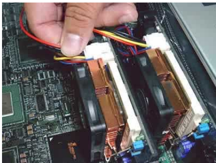
Connecting the power cable to the second PL-P3/SMP.
