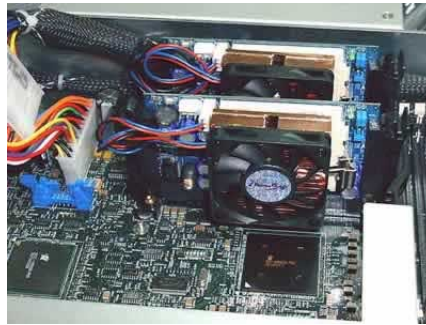
Inserting the second PL-P3/SMP into the processor slot.
