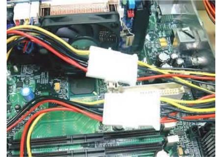
The connected cables for two PL-P3/SMPs.
