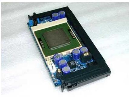
The PL-P3/SMP with installed processor.
