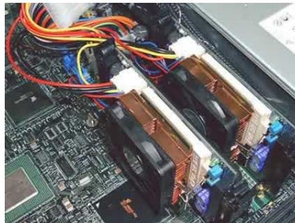
Dual PL-P3/SMPs, installed and connected.
