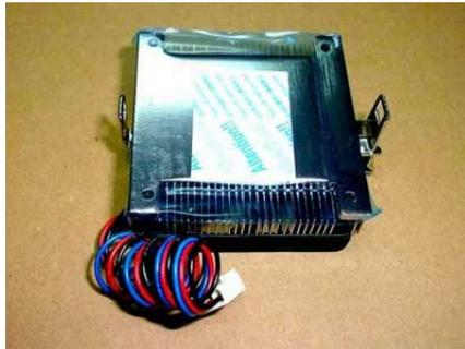
The PL-P3/Xeon-S's heatsink/fan (bottom view).
