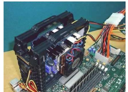
Dual PL-P3/Xeon-S's, installed and connected.
