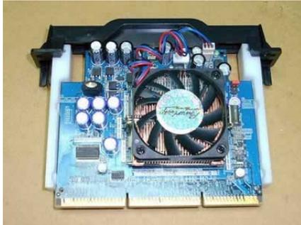
The PL-P3/Xeon-S after attaching the retaining bracket.
