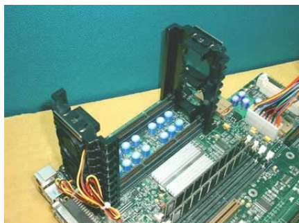
After removing both original CPUs.
