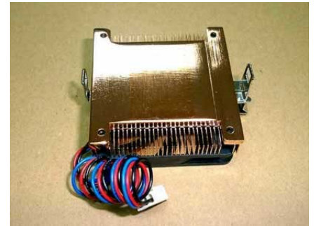
The PL-P3/Xeon-S's heatsink/fan (bottom view) after removing protective membrane.
