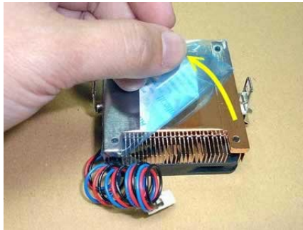
Peeling off the protective membrane.
