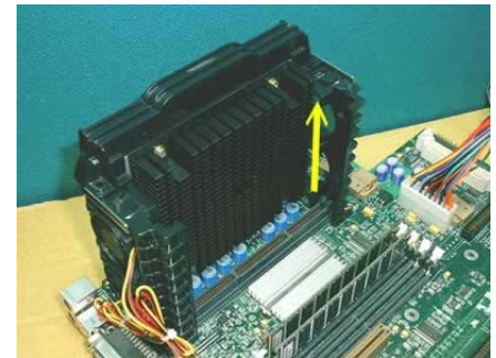
Removing the second processor. We recommend using a small brush to remove any dust from the slots.
