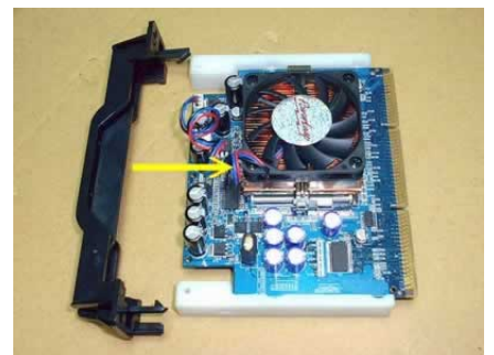
Attaching the retaining bracket to the PL-P3/Xeon-S.
