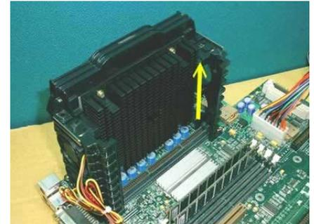
Removing the second processor. We recommend using a small brush to remove any dust from the slots.
