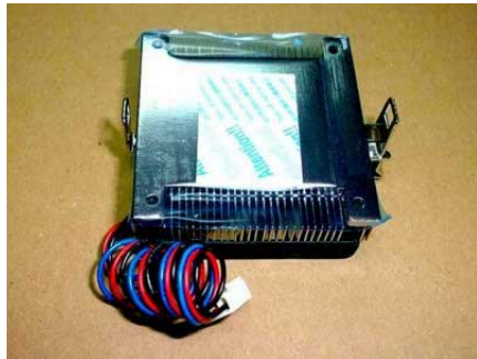
The PL-P3/Xeon-S's heatsink/fan (bottom view).
