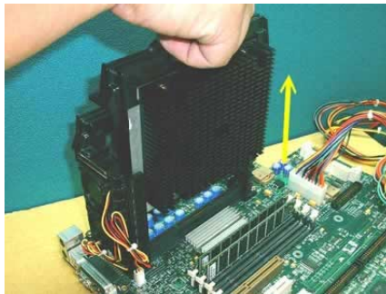
Removing the first processor (for details, refer to your motherboard manual).
