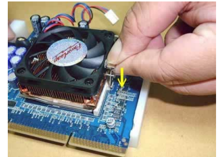
Attaching the heatsink/fan's retaining clip to the ZIF socket. (2)
