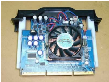
The PL-P3/Xeon-S after attaching the retaining bracket.
