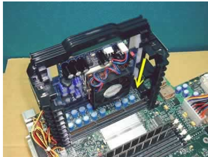
Inserting the first PL-P3/Xeon-S into a processor slot.
