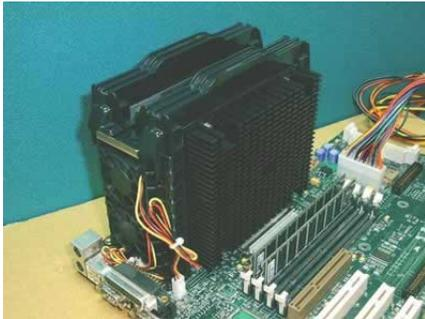
The original Slot 2 processors. Be sure to disconnect the system power before continuing with your processor upgrade.
