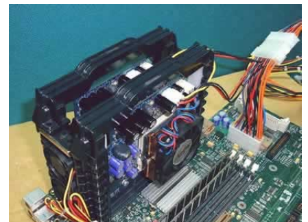
Dual PL-P3/Xeon-S's, installed and connected.
