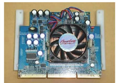
The PL-P3/Xeon-S after installing the heatsink/fan.
