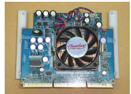
The PL-P3/Xeon-S after installing the heatsink/fan.
