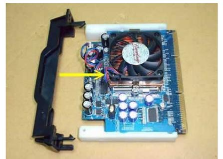
Attaching the retaining bracket to the PL-P3/Xeon-S.
