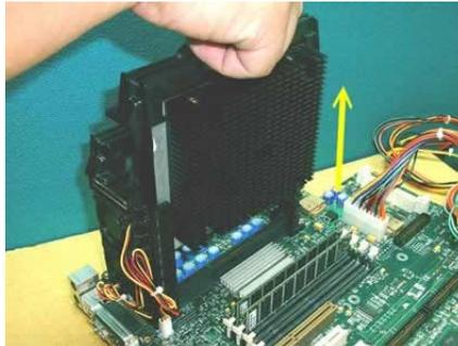
Removing the first processor (for details, refer to your motherboard manual).
