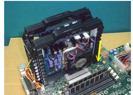
Inserting the second PL-P3/Xeon-S into a processor slot.
