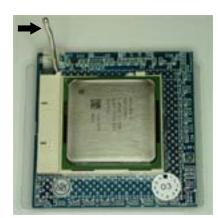
Using these landmarks gently seat the processor in the socket. Once it is firmly in place push down on the socket arm. Please follow the standard installation instructions from this point on.
