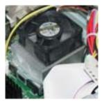
Locate the old processor. Remove the heatsink that is sitting on top of it. To do this you will need to remove the metal clips that are holding the heatsink in place.
