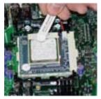
apply a thin layer to the top of the processor. This layer should cover the entire area, but does not need to be thick.
