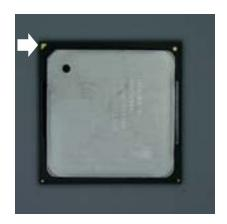
Locate the corner of the processor that has a gold colored triangle on it. Indicated by the white arrow.
