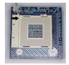
You will be lining up that corner of the processor with the notch in the socket. Indicated above by the black arrow.
