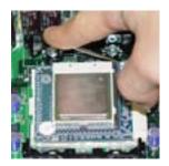
Insert the PL-P4/N into the socket. It will only fit in one way, so do not force it. Make sure the pins on the bottom line up with the holes in the socket. Then lower the lever in to place.
