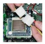
Now take the other end of the power cable and Tear open the tubette of Arctic Alumina and plug it into an extra system power cable. If you do not have an extra you can use the power cable to daisy chain off the CDROM.
