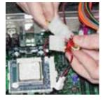
Connect the Molex Fan adapter to another free power connection or you may daisy chain of the PL-P4/N power cable.
