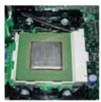
Lift the ZIF socket arm as far as you can. It should end up perpendicular to the motherboard. Then remove the processor.
