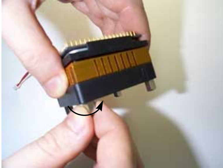
Figure 3. Tightening the hex nuts
