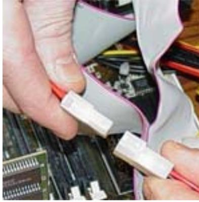
**6.** Plug the fan cable into the three prong end of the Molex Fan Adapter cable.
