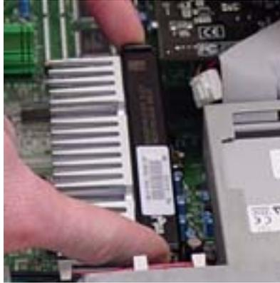
**3.** Take the SlotWonder unit and make sure the notch seen below lines up with the notch in the motherboard slot.
