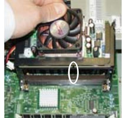
**4.** Slide upgrade in between retention rails until it is seated firmly. Push out on clips to lock into place
