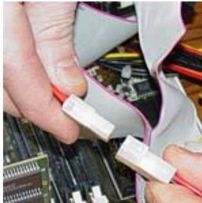
**6.** Plug the smaller end of the power cable into the PL-IP3/T
